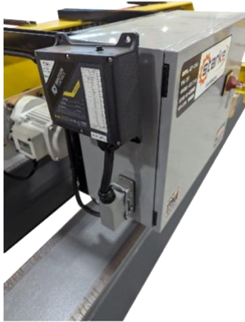
4.14.1 Radio Receiver Installed on Control Panel
