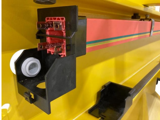
4.6.1 End of ElectroTrack System
