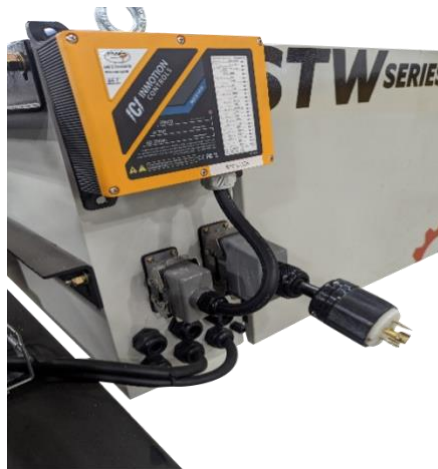
4.14.2 Radio Receiver Pre-Attached on Control Panel
