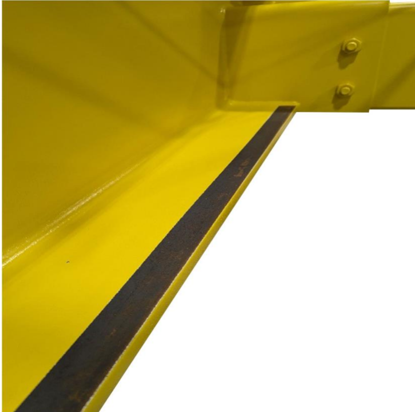
4.4.1 Taped Off Section on Crane
