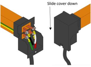
Image 7.13 Attached Wires
