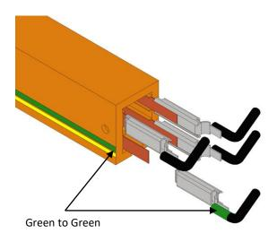
Image 1.2 Insert Conductor Couplers
