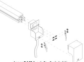
Image 7.14B Supply Box Exploded View
