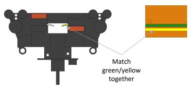
Image 7.15 Positioning Collector Trolley
