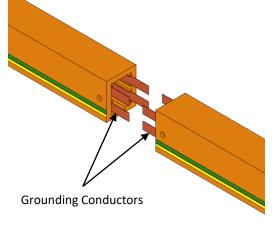
Image 1.1 Spaced Electrotrack
