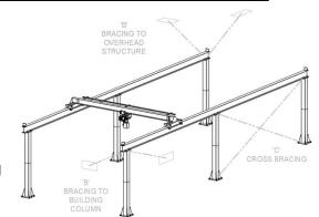
Diagram 8A. Examples of typical sway bracing locations.
