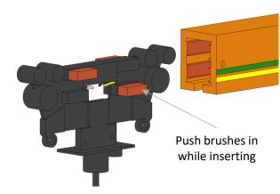
Image 7.16 Inserting Collector Trolley
