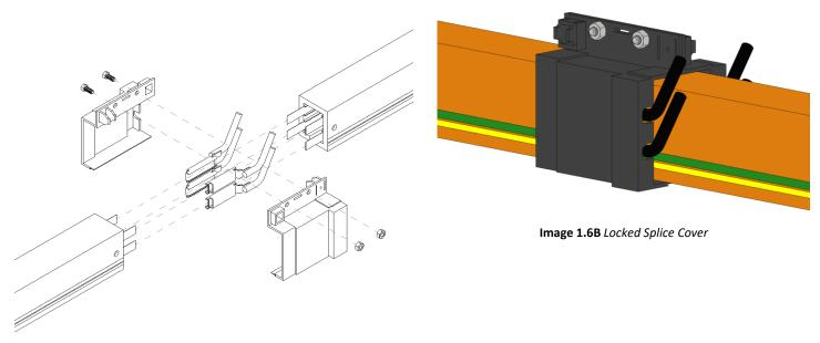
Image 1.6A Splice Cover Exploded View
