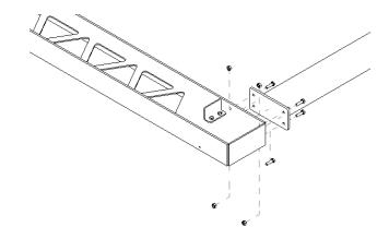
3. Once the legs are supported bring the upper beam over to the legs with a suitable lifting device like a forklift and bolt the beam to the leg assemblies using the hardware provided.
