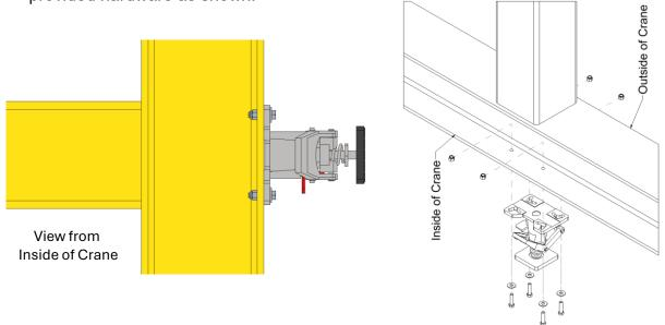
6. If casters are preassembled on your leg assemblies use caution to set the gantry in the upright position. Rolling casters can allow the gantry to move suddenly or the bottom of the gantry can roll away from the lifting device unexpectedly. Make sure, while lifting the gantry upper beam that the beam is chained or strapped to the forklift forks and forks are tipped back towards the forklift. If casters are not preassembled, bolt the casters to the end truck with the provided hardware as shown.
